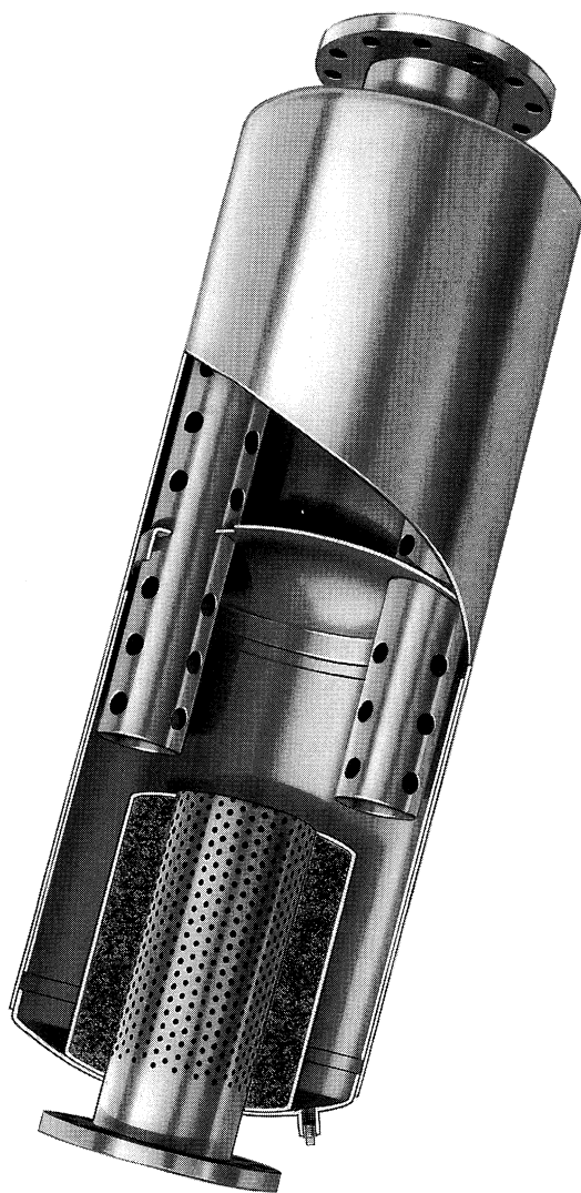
Figure 4-3. Basic UNIVERSAL SILENCER Combination-Type Silencer (Other Arrangements also Available)
