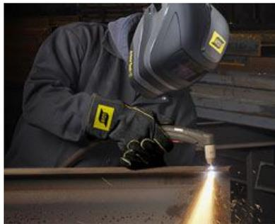
Fig. 57 - Corte a plasma, fonte - [www.esab.com.pt](http://www.esab.com.pt)
