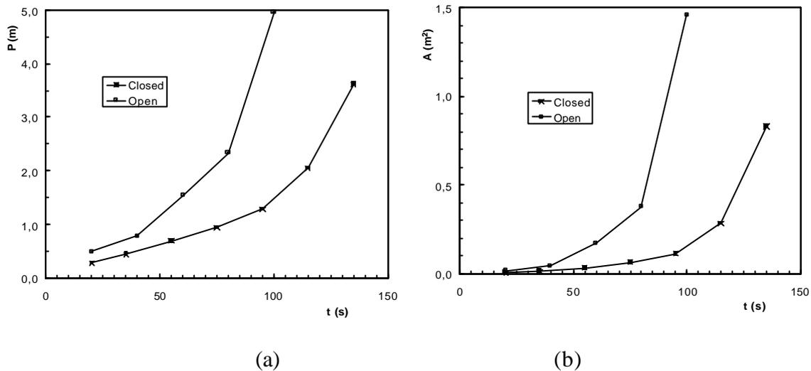
Figure 27 – Perimeter (a) and area growth (b) during tests with open and closed canyon.
