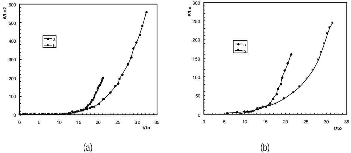
Figure 10 – Non-dimensional evolution of perimeter (a) and area growth (b) for fuels *a* and *b*, for a canyon:  $\alpha=22^\circ$  and  $\delta=21^\circ$ .
