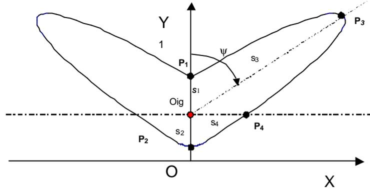
Figure 6 – Schematic presentation of fire shape given by the analytical model for a point ignition fire in a symmetric canyon
