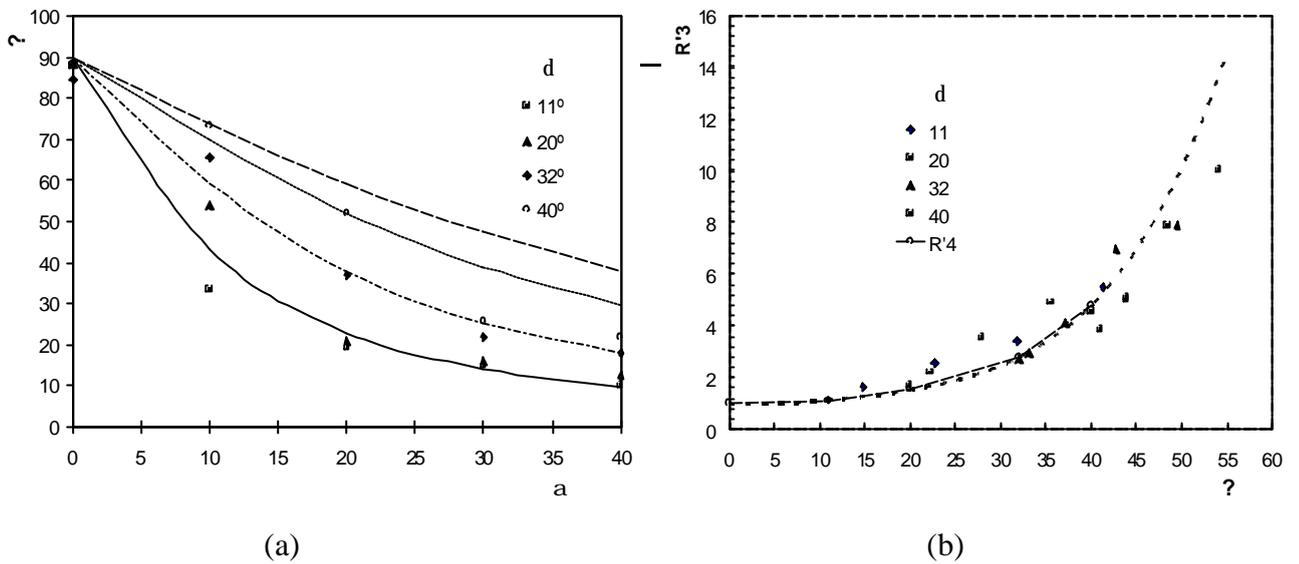
Figure 17 – (a) Direction of maximum spread compared with maximum slope direction  $\psi$ . The lines correspond to eq. [3]. (b) Non dimensional rate of spread  $R'_3$  as a function of the slope angle  $\theta$ . The dotted line corresponds to equation [6].
