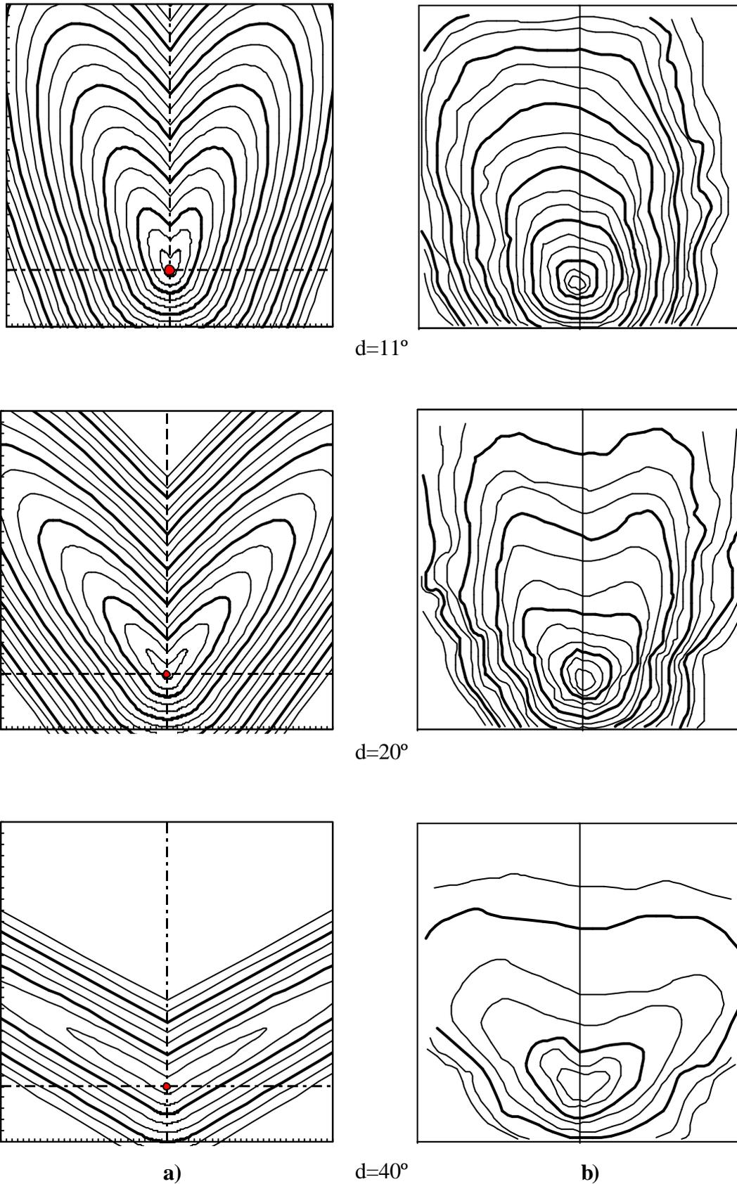
Figure 13 – Fire spread contours obtained in tests with  $\alpha=20^\circ$  for three values of  $\delta$ . Time step between bold lines is 60 seconds. (a) Analytical model; (b) Experimental results.
