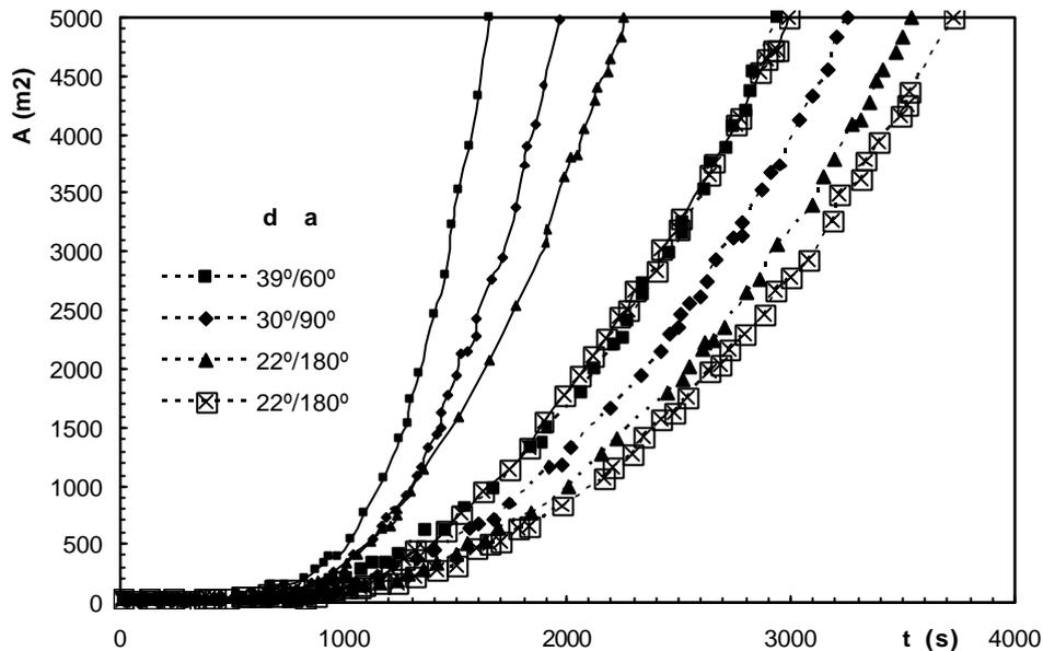
Figure 8 – Area growth in a canyon fire using static and dynamic simulations for four geometric configurations. The corresponding values of  $\delta$  and  $\alpha$  for each configuration are given in the legend. Dotted lines correspond to static model while full lines correspond to dynamic fire simulation.
