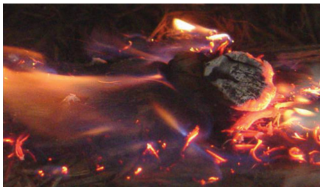
Fig. 4. Transition to flaming combustion in dried shredded hardwood mulch bed. Four ( d_0 = 50 \text{ mm} ) glowing firebrands were deposited.
