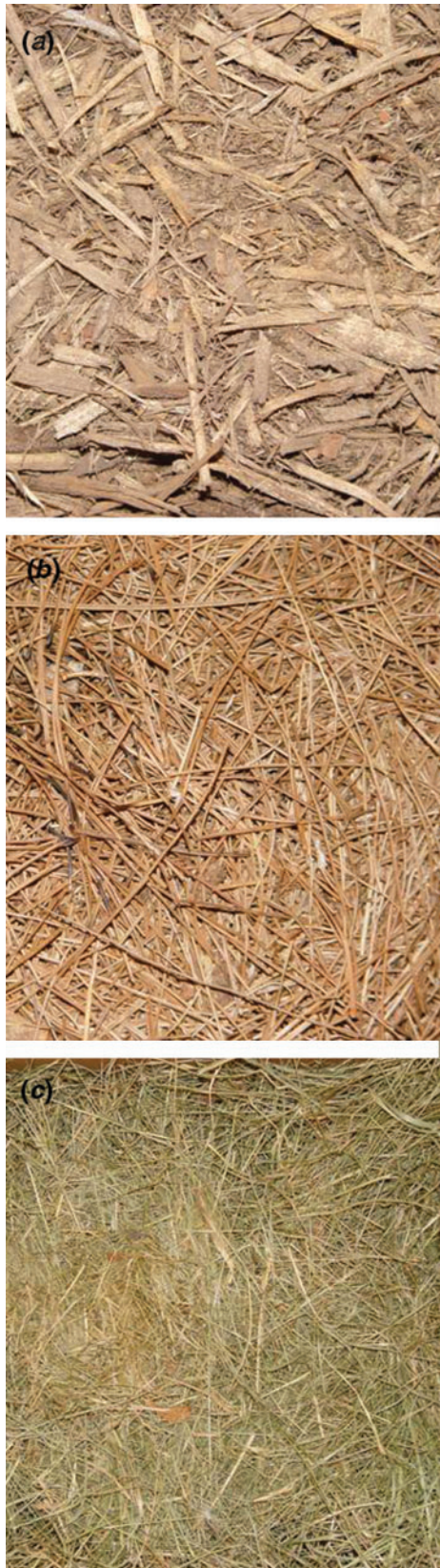
Fig. 2. Images of (a) shredded hardwood mulch, (b) pine straw mulch, and (c) cut grass used for the ignition experiments.
