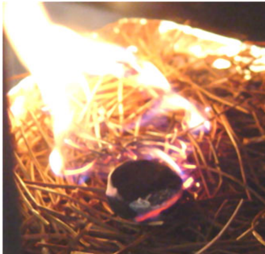
Plate 4. Single flaming firebrand which produced flaming ignition in a pine needle bed held at 11% moisture, d_0 = 25 mm.
