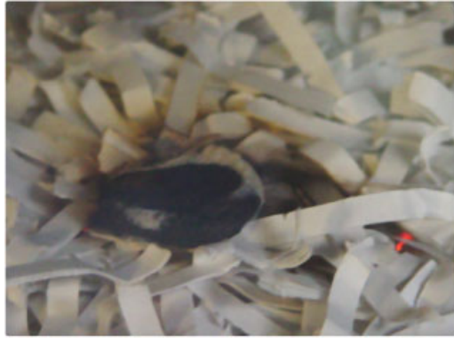
Plate 3. Single glowing firebrand which produced smoldering ignition in a shredded paper bed at 11% moisture content, d_0 = 25 mm.
