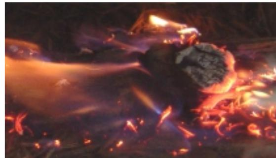
**Fig. 4 Transition to flaming combustion in dried shredded hardwood mulch bed. Four ( $d_0 = 50$  mm) glowing firebrand were deposited.**
