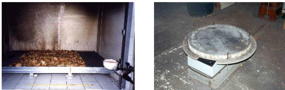
Figure 2. Experimental devices for the study of flammability of fuel beds
